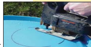
Jigsaw cutting the top hole
